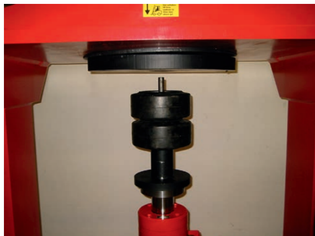
Preparation for mounting a steel banded solid
